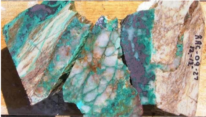
Drill RRC09-27 grading 11.12% Cu over 8.5 feet . Supergene chalcocite, copper pitch oxide rim, chrysocolla, malachite.
