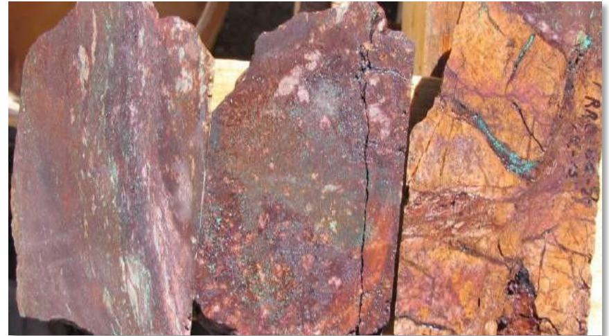
Drill RRC09-27; further oxidation of chalcocite to cuprite, copper "pitch" and malachite.
