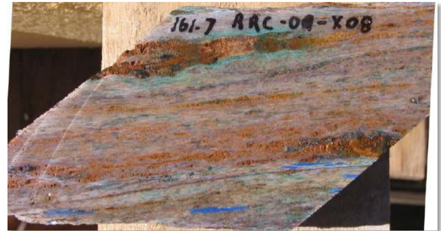
Drill RRC09-X08 from an interval grading 0.33% copper. Chrysocolla, azurite and minor remnant sulfides.
